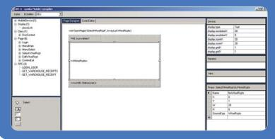
The integrated graphical development environment allows any required changes to be made quickly. As soon as the change is activated it is immediately available to all mobile staff. Installation of such changes into the individual smartphones is not required – data and the application are always current.
